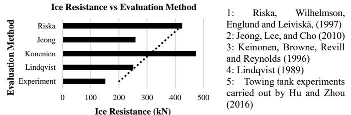
Fig. 7: Ice Resistance evaluated using different methods and experiments.
