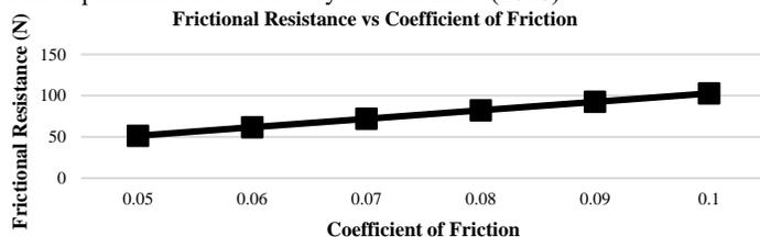
Fig. 9: Frictional Resistance component and its dependence on skin friction coefficient. (ITTC resistance formula (2002) (Ittc.info, 2018).
