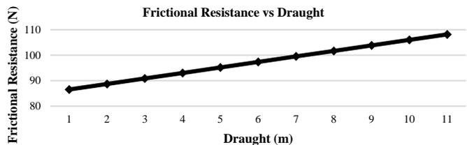
Fig. 13: Frictional Resistance and its dependence on draught (ITTC resistance formula (2002) (Ittc.info, 2018).
