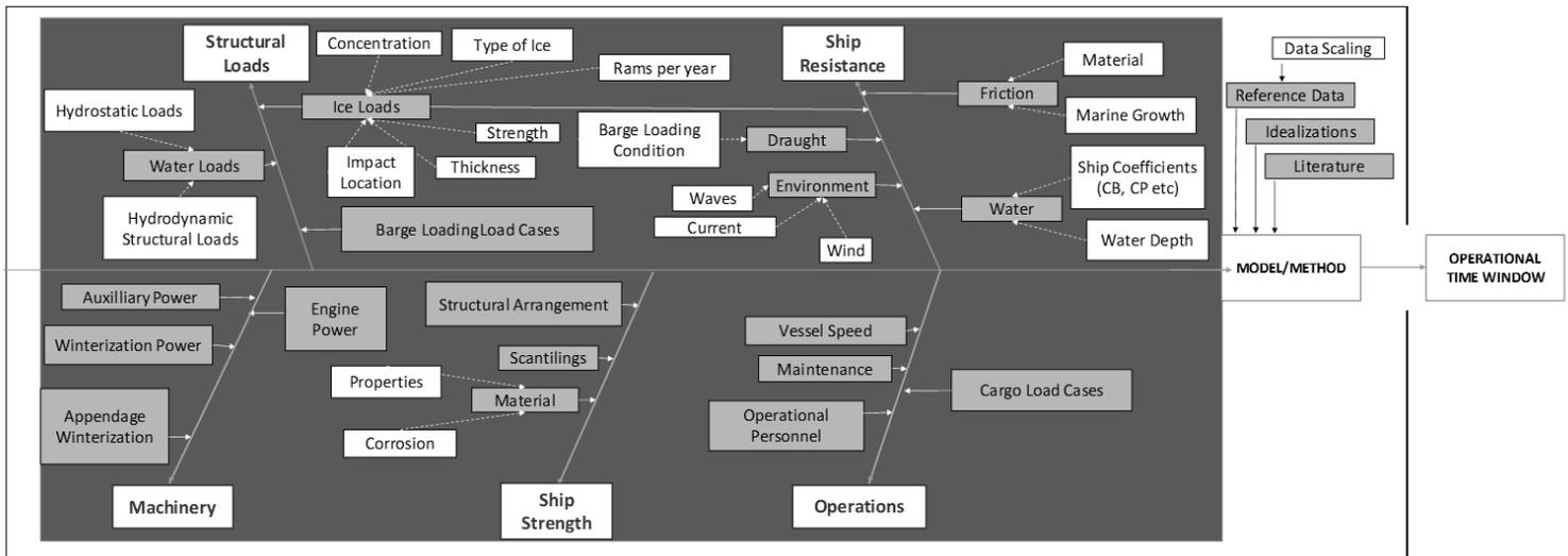
Fig. 1: Fish bone diagram depicting influence of different variables on the Operational Time Window for a barge. Area enclosed by grey box represent primary, secondary and tertiary dependencies influencing OTW. White boxes with bold alphabet represent primary criteria. Grey boxes represent secondary criteria while white boxes represent tertiary criteria. Influence on OTW by these dependencies depends on by efficiency of Method/Model box used to assess these.
