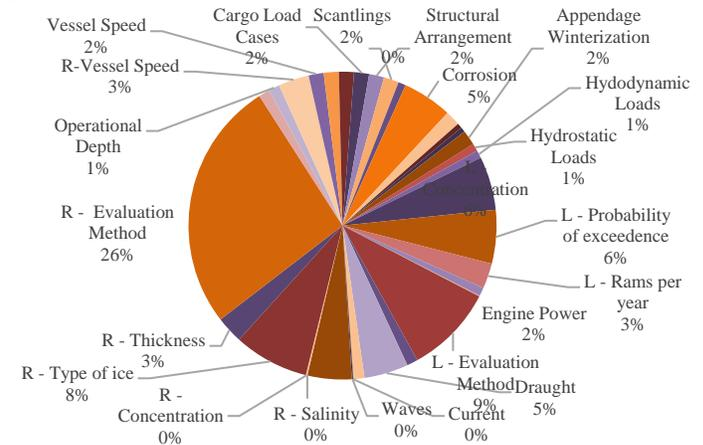
Fig. 3: Pie chart of uncertainty contributions of all criteria in Fig. 1 using Basic VMEA (R denotes criteria under Ice Resistance and L denotes criteria under Structural Loads due to ice).
