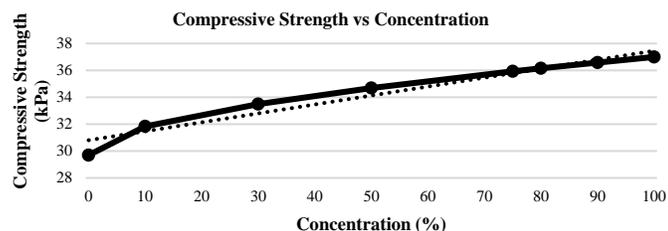
Fig. 14: Compressive strength of ice and its dependence on ice concentration (Kujala, 1994).
