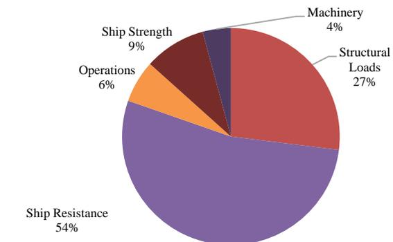
Fig. 4: Pie chart of uncertainty contributions from primary criteria in Fig. 1 using Basic VMEA.
