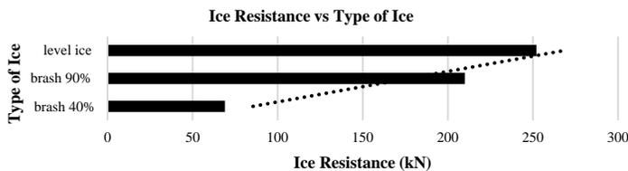
Fig. 8: Ice Resistance evaluated for different types of ice based on towing tank experiments carried out by Hu and Zhou (2016).
