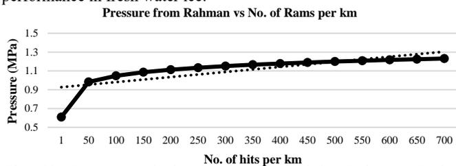
Fig. 12: Pressure calculated using method by Rahman, Taylor, Kennedy, Simões Ré, and Veitch (2015) for different rams per km.
