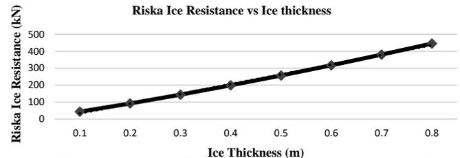
Fig. 6: Distribution of Ice Resistance for varying ice thickness (Riska, Wilhelmson, Englund and Leiviskä, (1997).
