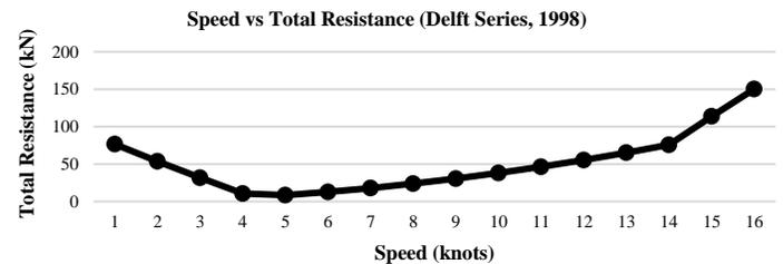
Fig. 10: Total Resistance and its dependence on velocity using Delft series. (Delftship.net, 2018).
